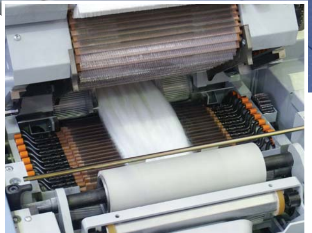
Drafting head with a light moving assembly
